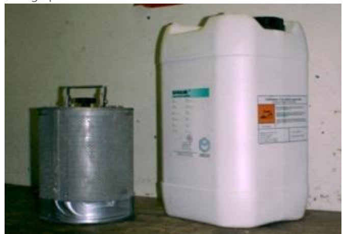
Bell scrubber canister and drum of CO 2 absorbent
