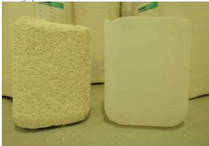
CO 2 absorbent after time at depth within a sealed container.
