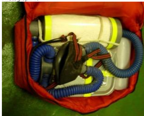
SP2 Personal scrubber and thermal regenerator
