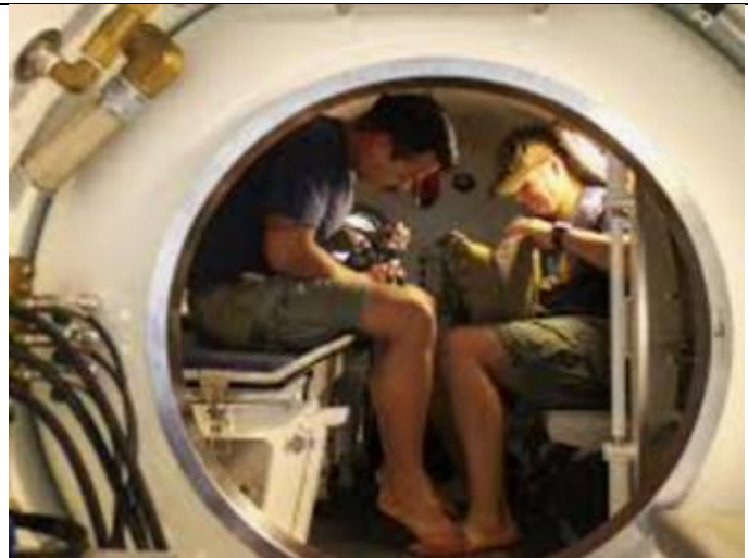
The reality of an IMCA compliant two-person two-compartment chamber
