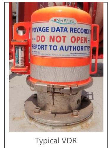
The data is stored on the Voyage Data Recorder (VDR). The length of the ship denotes the capacity and type of monitoring. The VDR is very similar to an aircraft's 'black box'. It stores the data typically for 30 days and either floats off the vessel or is ROV retrievable.
