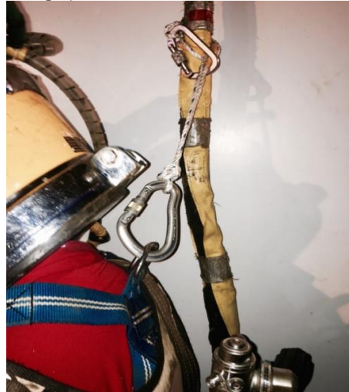
Rescue lanyard used to align IP to trunk
