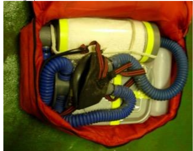
SP2 Personal scrubber and thermal regenerator
