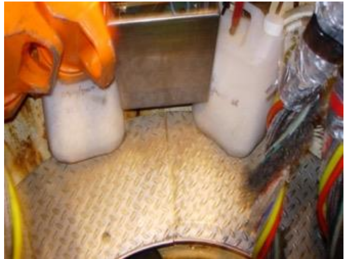
CO 2 absorbent inside a bell (Juice containers)
