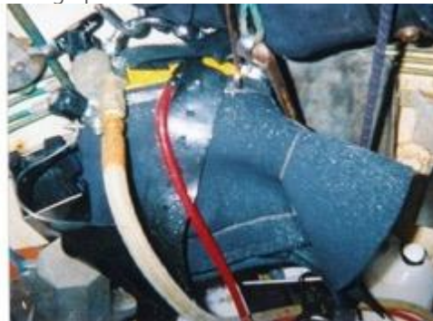
CO 2 dust on bellman's breathing equipment below scrubber
