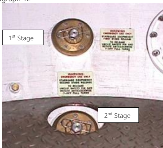
1 st & 2 nd stage release with divers umbilical removed Note: Different bell designs have different layouts
