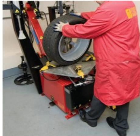
Figure 37 Tyre-changing machine with integrated wheel lift
