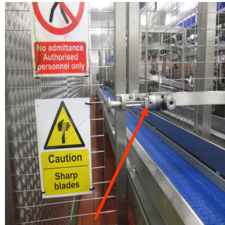
Castell Type key restricted access to fenced area
